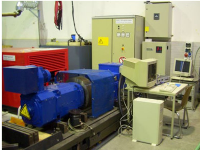
Figure 129: The 80 kVA machine unit as replica of a wind energy plant
