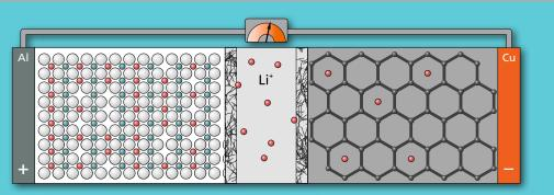
Principle of a Lithium Ion Battery
