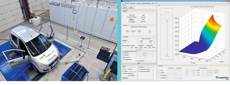
Simulation and "Hardware in the Loop" tests play an important role in modern development processes, since they promise significant time and cost savings. This applies also to the area of electrical systems, where storage devices, such as Lithium Ion batteries often are a key component. For such applications Fraunhofer IWES offers a detailed simulation model known as ISET-LIB.
