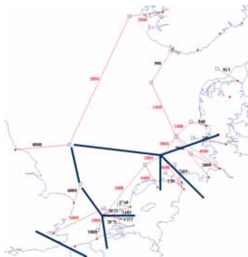
Figure 2: Meshed offshore network in the North Sea, interconnecting approximately 100 GW offshore wind farms, with direct extensions to mainland (bold dark blue lines). Source: TradeWind.
