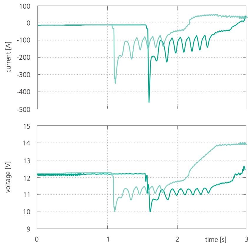
*Virtual starter battery with ISET-LAB-RT: Two different ignition procedures of a conventional car using a real battery (light green) and a virtual battery (green). The matching of the dynamic behaviour is clearly demonstrated.*
